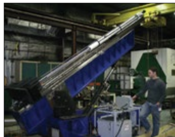
Convertible Test System 20,000 lb load - 100" CC
